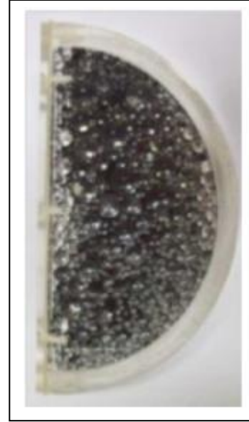
Fig. 3. A physical phantom dedicated for 2D and 3D breast imaging [7]
